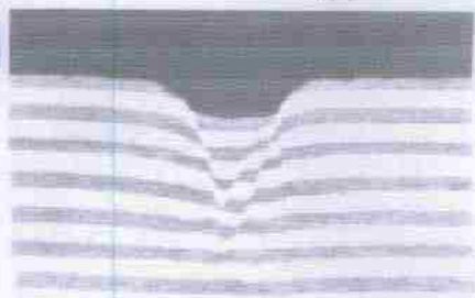
Fig. 3.6 Failure shear failure pattern under a rectangular footing on the surface of loose sand ( ID_r = 15\% ). (From De Beer and Vesic, 1968.)
