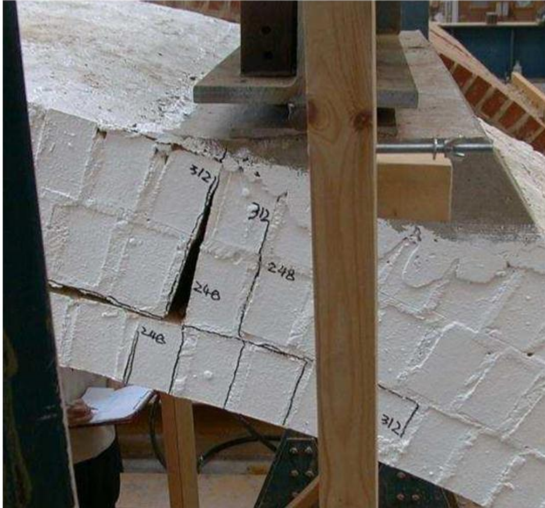
Figure 5. Hinges forming in the arch barrel at \frac{1}{4} span (left) and \frac{3}{4} span (right).
