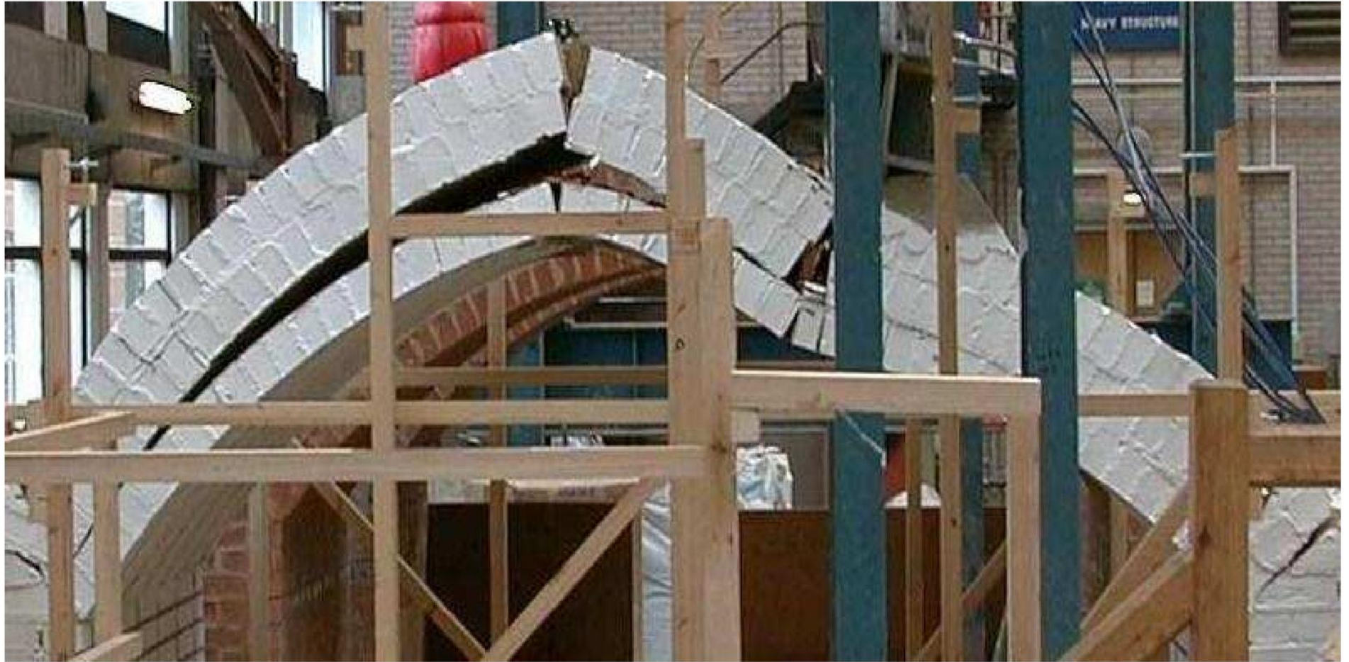
Figure 4. A reinforced arch (arch 2) without shear reinforcement showing premature
