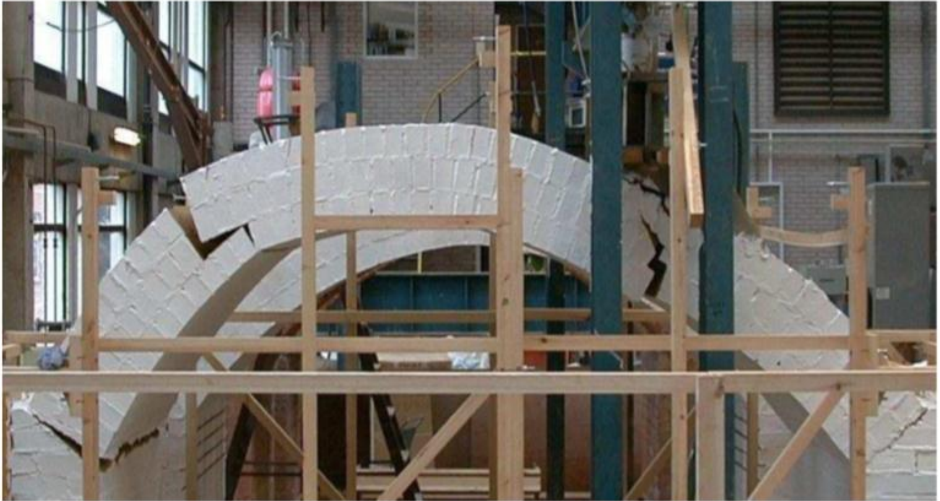
Figure 3. Arch 1 (unreinforced control) showing the 4-hinge collapse mechanism.
