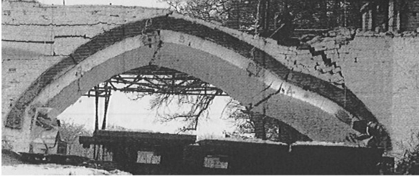
Fig. 7. The Prestwood bridge: the collapse mechanism.
